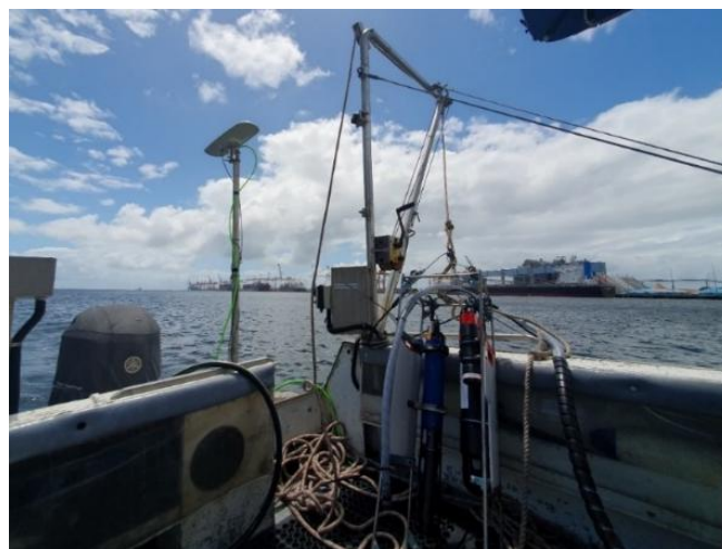
Figure 2.1 Plume monitoring equipment setup including the ADCP mounting pole, and the profiling array including the co-located LISST, YSI and pump sampler frame (BMT 2023).
